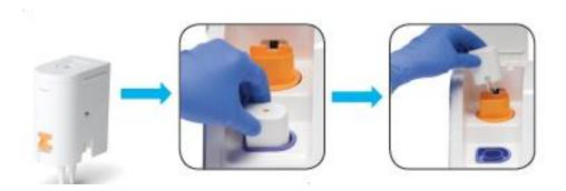
12. Lift the **White Transfer Cartridge** out again and push it firmly into the **Orange test Base** at the back of the analyser to connect them. The orange indicator will depress to the bottom to dispense the sample.
